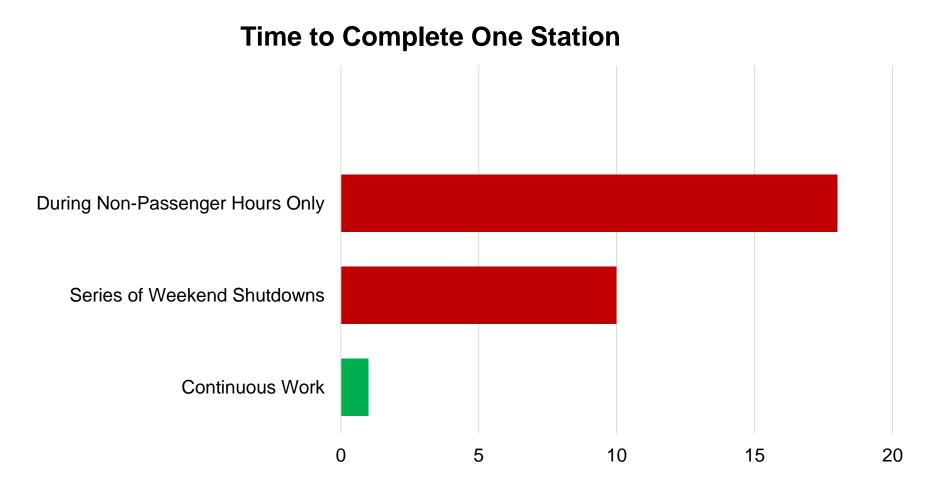
Providing 24/7 track access substantially reduces project duration, is safer, and costs less
